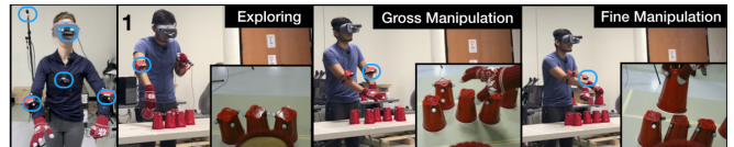
Fig. 1: The cameras in VR telepresence task simulate the cameras equipped on a tele-presence tele-action nursing robot [4]. Participants typically executed exploring, gross manipulation (reaching, carrying), and fine manipulation (grasp, place) actions to complete the cup-stacking task.
