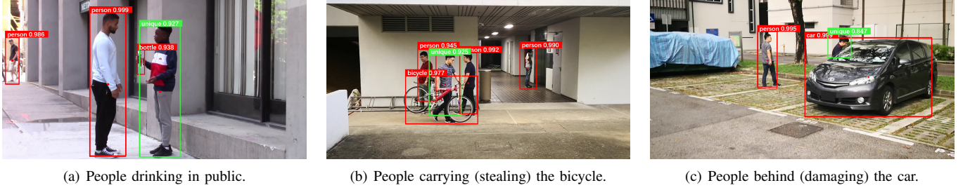
Fig. 2. Three different outdoor scenarios for unique role recognition. The green bounding box is the recognized unique target in the scene.
