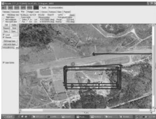
Figure 2. Ground Station Operator Interface showing flight plan and actual UAV position (August 2003, Fort Benning, Georgia).
